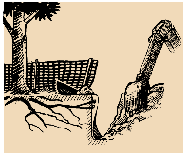
Figure 26. When digging near trees suitable for preservation, the first cut should be made by hand labor with shovels under supervision of an arborist. Exposed roots should be neatly cut with a sharp saw. To protect them from drying out, the ends of severed roots can be covered with a plastic sandwich bag held in place by a rubber band.
