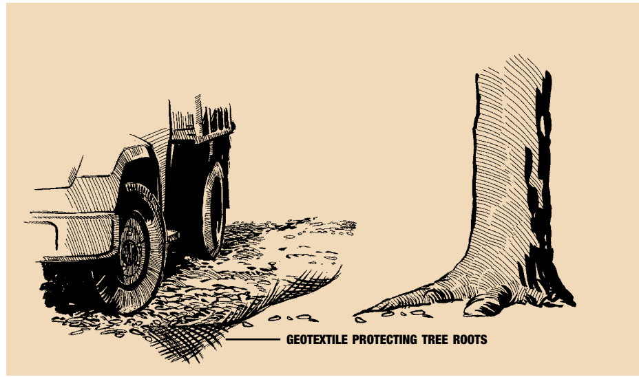
Figure 23. Two to 4 inches of mulch placed on a geotextile sheet protects soils from compaction caused by construction equipment and material storage.
