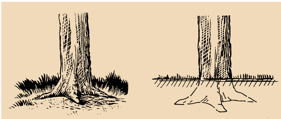
Figure 20. Do not raise the natural soil level within a TPZ. Trees that have been buried in fill can be identified by a lack of root flare.
