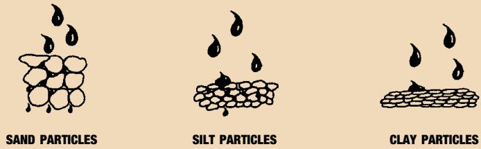
Figure 5. The amount of sand, silt, and clay particles found within a soil make up a soil's texture. Structure is how these particles are grouped together.
