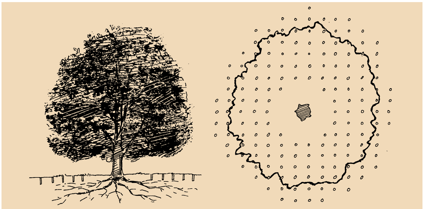
Figure 30. Vertical mulching can help repair compacted soils and help trees recover from root systems damaged by compacted soils and root removal.
