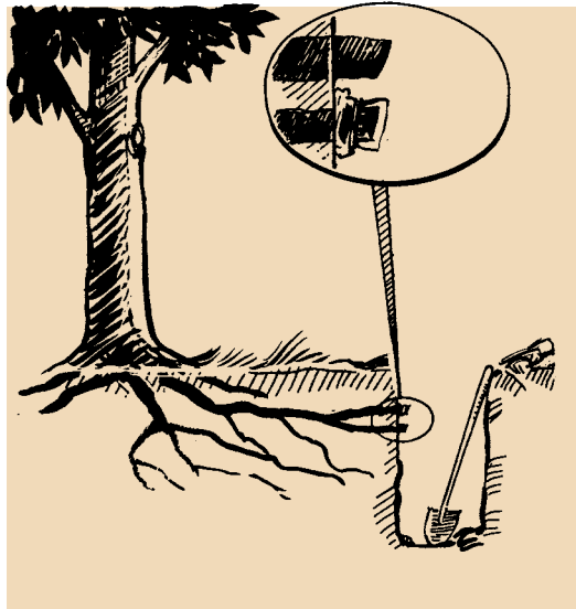
Figure 26. When digging near trees suitable for preservation, the first cut should be made by hand labor with shovels under supervision of an arborist. Exposed roots should be neatly cut with a sharp saw. To protect them from drying out, the ends of severed roots can be covered with a plastic sandwich bag held in place by a rubber band.
